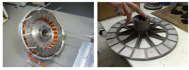
c) Assembled stator
