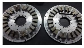
a) Two stator parts
