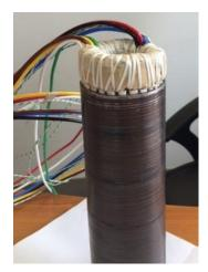
Figure 7. Stator of the fault tolerant double-star PM machine.
