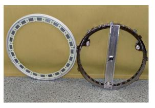
b) Rotor and stator
