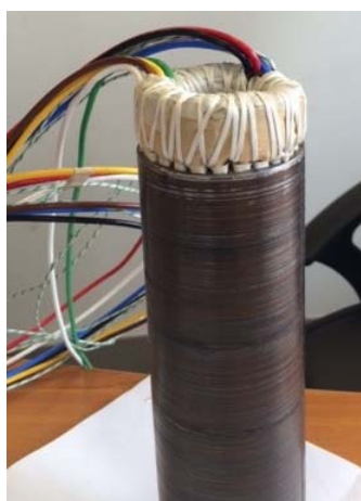
Figure 7. Stator of the fault tolerant double-star PM machine.
