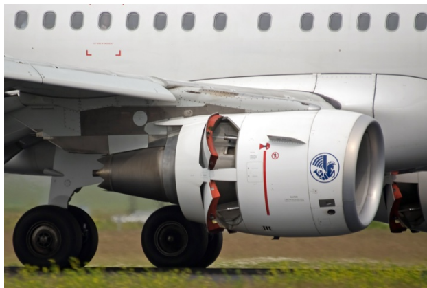
Figure 6. Thrust reversers deployed on the CFM56 engine of an Airbus A320.
