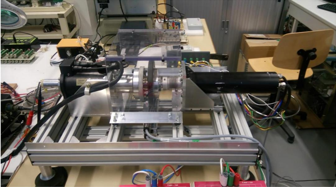
Figure 8. Test bench of the fault tolerant double-star PM machine.
