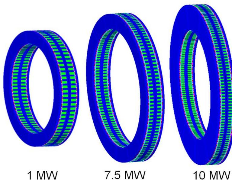
Figure 11. Axial field PM generators for wind turbines.
