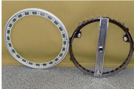
b) Rotor and stator
