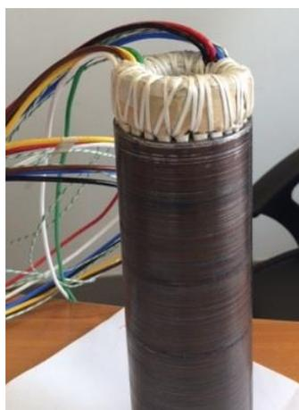
Figure 7. Stator of the fault tolerant double-star PM machine.
